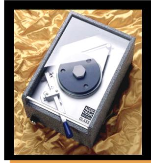
Audio Desk System is a motorized cutting device manufactured in Germany. It is designed to "true" the shape of the CD to reduce mechanical jitter, and also trims the edge of the CD to a 38° angle to reduce laser scatter. This edge is then further treated with a black marker. The process takes about 60 seconds and results in pronounced improvements in focus, transient attack, detail and transparency.
